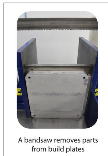
A bandsaw removes parts from build plates
